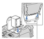
Align the battery with the groove.
